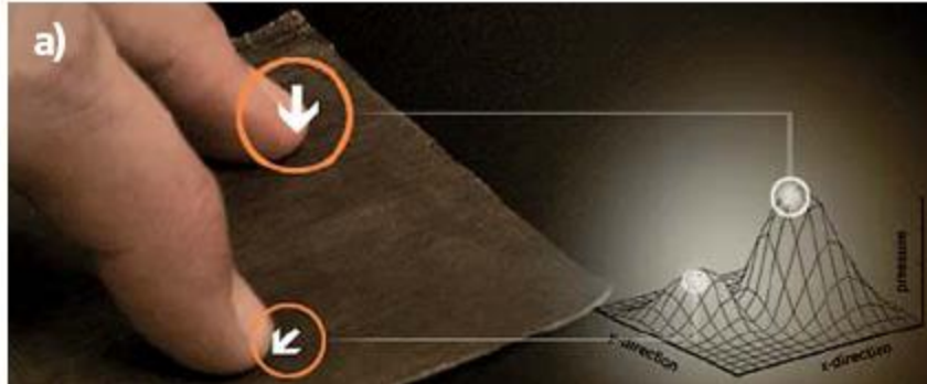
(a) TactArray, a flexible capacitive array tactile sensor from Pressure Profile Systems, Inc., is appropriate for sensing contact locations and areas under sliding conditions.
