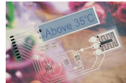
Printed sensors: Unique sensing labels – based on printed electronics- bring new functionality and crystal clear reads to temperature controlled supply chains.
