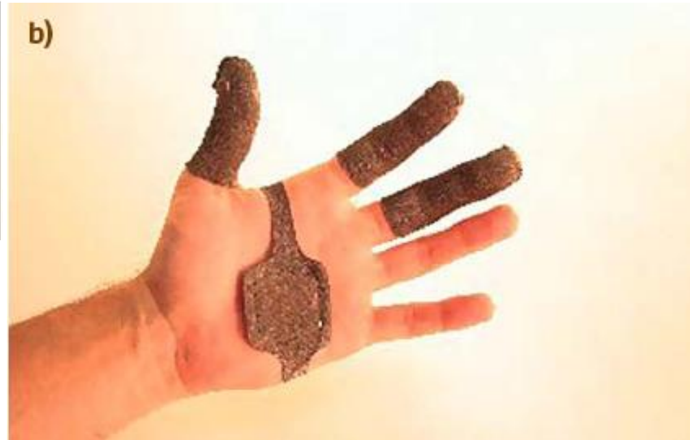
(b) Conformable TactArray sensors can fit on a human or robotic hand (courtesy Pressure Profile Systems, Inc.)
